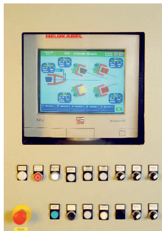
Standardised process control and visualisation of an extrusion system at our Windsbach factory.
